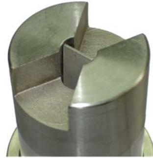
Fig. No.1 Photograph of one of the sensors Fig. No. 2 - Sensor fitted in a BOSS having passages
